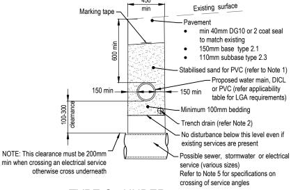
TYPE C - UNDER **CARRIAGEWAY (SEALED)**  Approved excavated material placed and compacted in layers and tested as per specification Undisturbed ground
